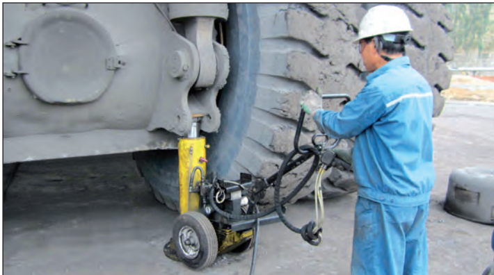
▼ Enerpac POW'R-RISER® used in mining operations to lift heavy equipment.
